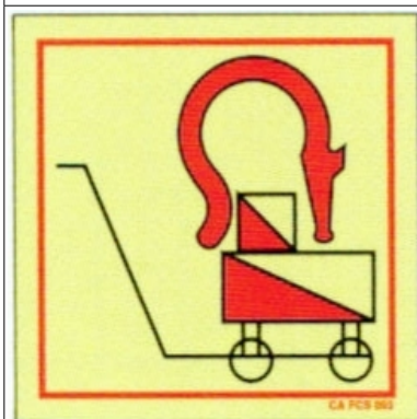
Pompa antincendio carrellata Movable extinguisher pump
